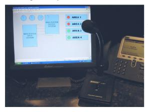
There are many different types of zoned audio systems to choose from. These range from the basic, bush button select a source for each zone system, to the advanced computer programmed digital matrix systems which can be fully automated and controlled via touch screen. We can provide a solution for you that enables to routing power to give your system the flexibility when needed but more importantly the easy of use that most end users require.
